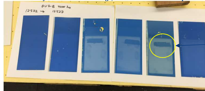
PVDF or acrylic waterborne coatings, 4000 hours UVB-313 exposure:
