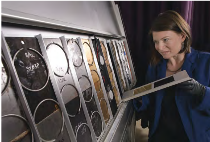
After thousands of hours in an accelerating weathering apparatus, metal panels treated with the new protective coating system were analyzed by Dr. Lasseter Clare for any film degradation. Photo courtesy of www.brucemacgregorphotography.com .
