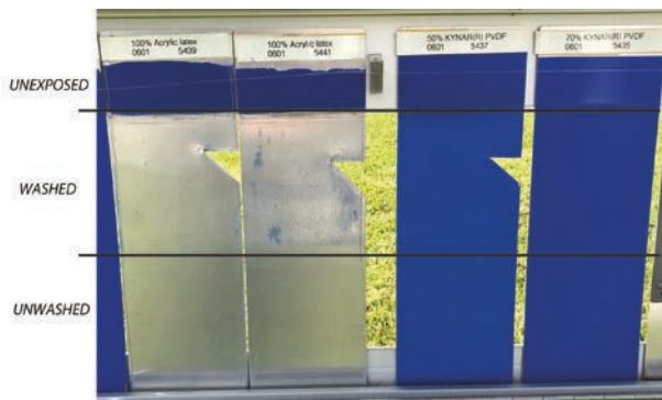
Photo of a cobalt blue natural weathering study taken on August 12, 2018, after weathering in south Florida for more than 17 years. From left to right, the first two panels are 100 percent acrylic latex, approved by Master Painters Institute (MPI) 311, Latex, Exterior, High Performance Architectural, Semi-Gloss , and now eroded and no longer on the test panel, followed by 50 percent PVDF-acrylic (American Architectural Manufacturers Association [AAMA] 2604, Voluntary Specification, Performance Requirements and Test Procedures for High Performance Organic Coatings on Aluminum Extrusions and Panels [with Coil Coating Appendix] ), and 70 percent PVDF (AAMA 2605, Voluntary Specification, Performance Requirements and Test Procedures for Superior Performing Organic Coatings on Aluminum Extrusions and Panels [with Coil Coating Appendix] ).
